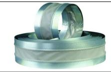
Flexible Connector prevents vibration and noise to transfer the galvanized duct which carries air in heating ventilation systems. The material which is placed between two galvanized sheet is locked with multi lock system. Never seperates each other.
