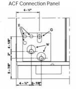
G Gas connections Ø 1/2" FPT W Water connections Ø 1" FPT E Electrical knockouts Ø 7/8" FPT
