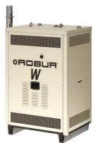
**GAHP-W** - Cooling capacity up to 4.5 tons and heating capacity up to 132,400 BTU/h nominal output (95,500 BTU/h input) while supplying hot water up to 149 °F. 139% heating efficiency at nominal conditions.
