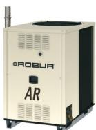
**GAHP-AR** - Reversible absorption cooling cycle with 126% heating efficiency at nominal conditions. The reversible absorption heat pump is a gas fired unit providing approximately 5 tons of cooling. Chilled water down to 37.4 °F is possible. In the heating mode hot water up to 140 °F is possible providing 120,400 BTU/h nominal output (95,500 BTU/h input). This unit uses outside air for heat rejection in the cooling mode and outside air as a heat source in the heating mode.
