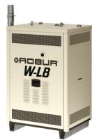
**GAHP-W LB** - Cooling capacity up to approximately 4 tons and heating capacity up to 119,400 BTU/h nominal output (95,500 BTU/h input) while supplying hot water up to 140 °F. 125% heating efficiency at nominal conditions.
