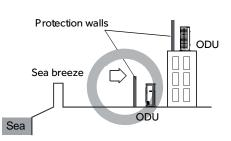
• A protection wall should be constructed with a solid material such as concrete to block the sea breeze and the height and the width of the wall should be 1.5 times larger than the size of the outdoor unit. Also, secure over 28 in (700mm) between the protection wall and the outdoor unit for exhausted air to ventilate.
