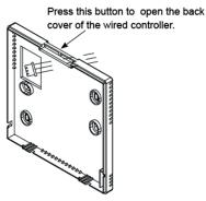
1. P ut communication wire through the hole in the back  $% \left( {{{\rm{cover}}}} \right)$  cover as sho wn.
