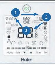
The wired controller will momentarily display all display icons upon powering up or when resetting the system.
