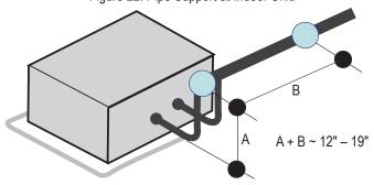
Figure 23: Typical Pipe Support Location—Change in Pipe Direction.
