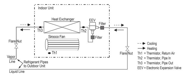
Figure 6: High-Static Ducted B8 Refrigerant Piping Diagram
