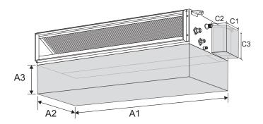
Figure 17: Low-Static Built-In Ducted (B3, B4) Indoor Unit Maintenance Clearances.
