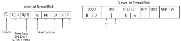
Figure 39: Location of Power Wiring and Communications Cable Terminals in the Vertical/Horizontal Air Handler Unit
