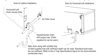
Figure 29: Vertical / Horizontal Air Handler Unit U-Trap Specifications.
