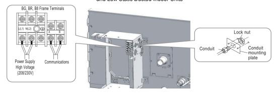
Figure 35: Terminal Block in the High Static (BH, BG, BR, B8 Frame) Ducted Indoor Units
