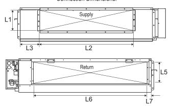
Figure 13: Low-Static Ducted (L1/L2/L3) Indoor Unit Duct Connection Dimensions.
