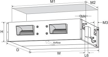
Figure 10: Low-Static Ducted Indoor Unit Dimensions.
