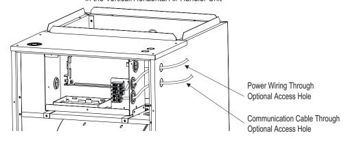
Figure 40: Terminal Block in the Vertical / Horizontal Air Handler Units
