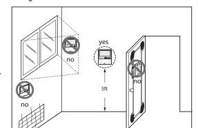
Figure 51: Wired Remote Controller Installation
