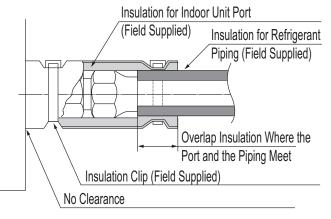
Figure 25: No Air Gap in Pipe Insulation to Indoor Unit Frame.
