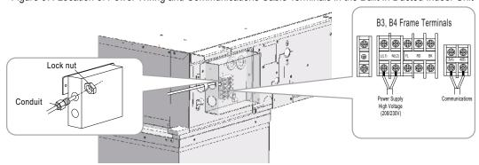
Figure 38: Terminal Block in the Built In Ducted Indoor Units
