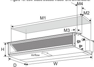
Figure 11: Low-Static Ducted Indoor Unit B3/B4 Dimensions.
