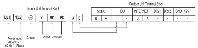
Figure 36: Terminal Block in the Low Static (L1, L2, L2 Frame) Ducted Indoor Units
