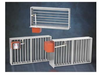
The MST motor powers the damper open and closed and is designed to operate in all weather conditions. The AOBD is recommended for low pressure duct systems, less than 0.75'' S.P. For higher pressure systems use the Comfortron<sup>TM</sup> series of dampers.
