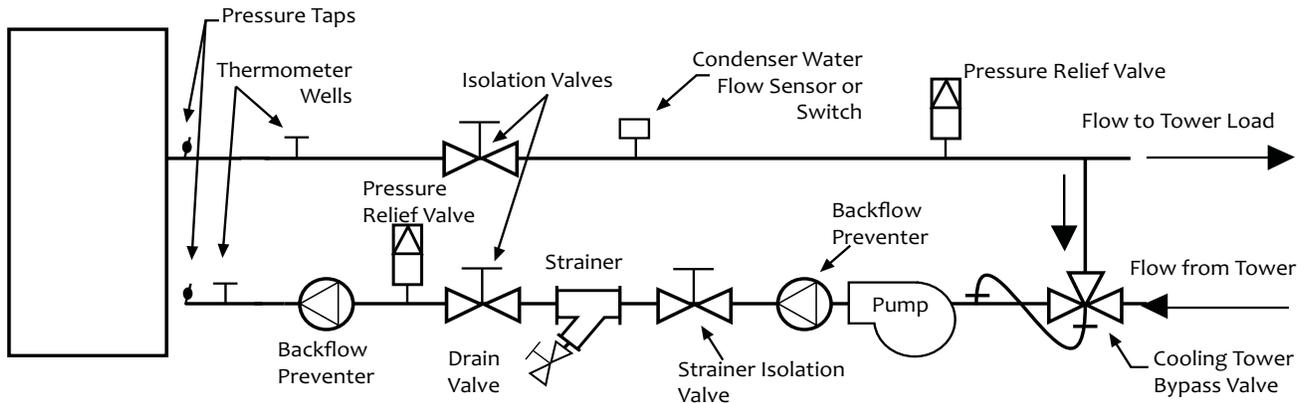
Note: Only required for equipment without motorized condenser valves.
