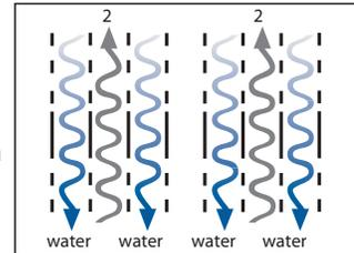
The same results are achieved if circuit 1 is ran and circuit 2 cut out; optimum heat transfer, even at part-load.
