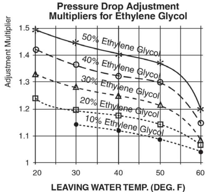
**Note:** Correction factors shown above are to be applied to Std. Product Data chiller pressure drop curves for straight water.
