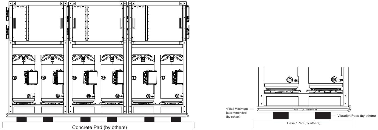
**Note:** Size and weight distribution is to be determined by a qualified structural engineer per individual job requirements.
