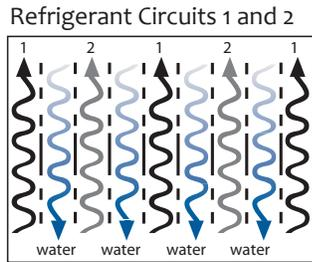
If circuit 1 is cut, the unique design allows each water channel to remain in contact with refrigerant circuit 2, providing optimum heat transfer.
