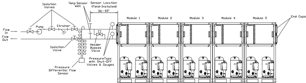
Figure 20 - Field Piping Reverse Return
