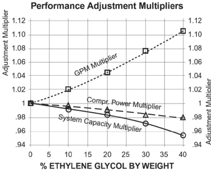
**Note:** Correction factors shown above are to be applied to Std. Product Data @ ARI 550/590 44°F. Leaving Chilled Water / 85°F Entering / 95°F Leaving Conditioned Water.
