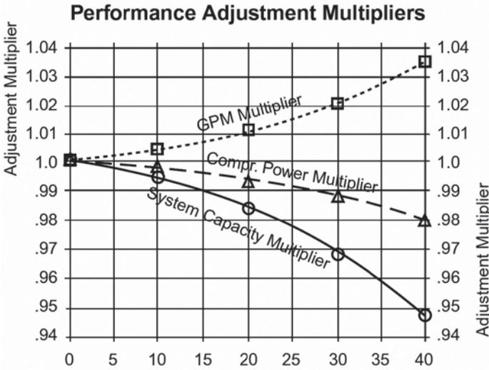
**Note:** Correction factors shown above are to be applied to Std. Product Data @ ARI 550/590 44°F. Leaving Chilled Water / 85°F Entering / 95°F Leaving Conditioned Water.
