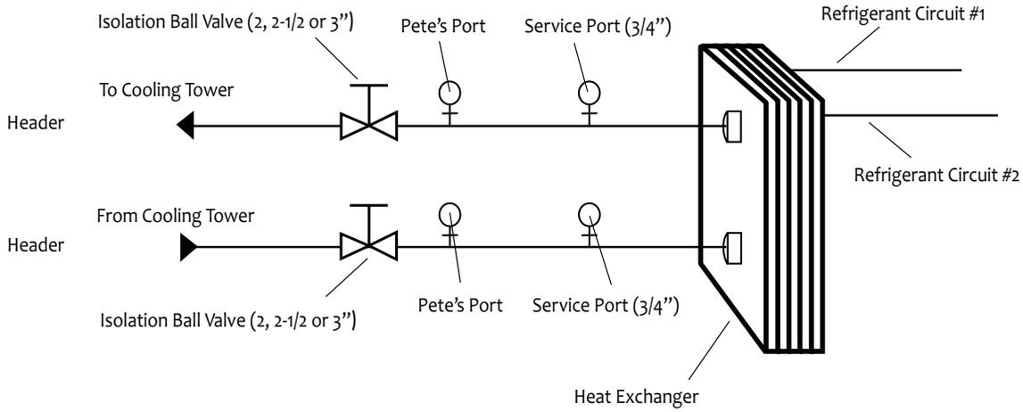
**Figure 22 - Chilled Water Circuit**
