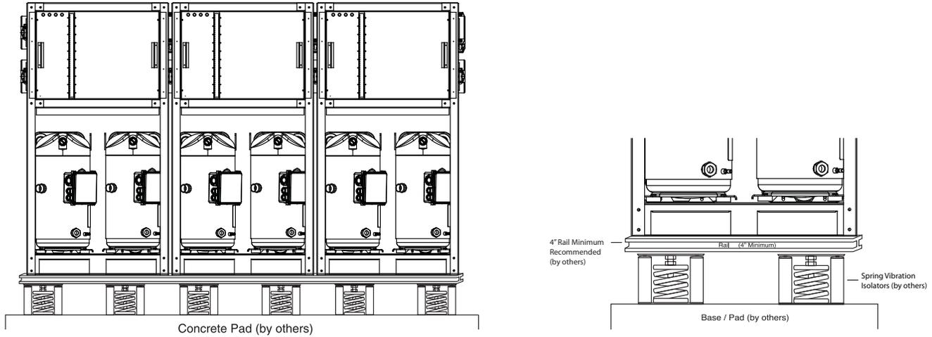
**Figure 5 - Vibration Isolation Pads Option**
