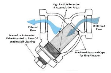
Figure 34: WYE Strainer - Flanged Ends
