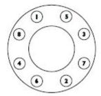
Note: Excessive bolt torque may damage flanges. Please refer to established flange bolt torques for guidelines.
