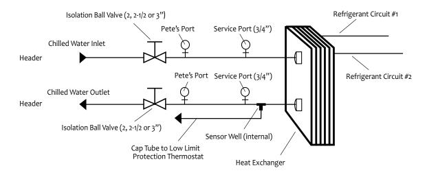
Note: Figure 21 and 22 depict hydronic piping in each ClimaCool chiller module and are shown with water isolation valves.
