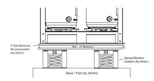
Figure 5 - Vibration Isolation Pads Option
