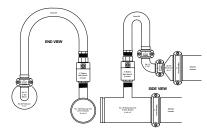
Figures 19 and 20 on page 16). The purpose of the chiller/heater system bypass is to prevent deadheading of the pumps when all of the internal unit valves go closed as well as allow temperature and differential pressure sensors to sense active flow. The bypass should be sized for an absolute minimum of one module's worth of design flow. Please refer to selection submittals for design flow rates.
