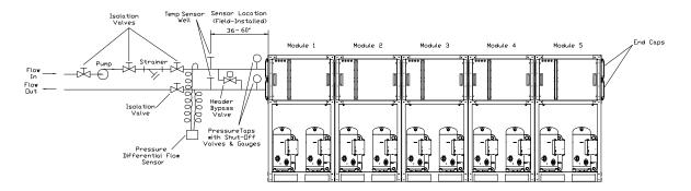
Figure 20 - Field Piping Reverse Return
