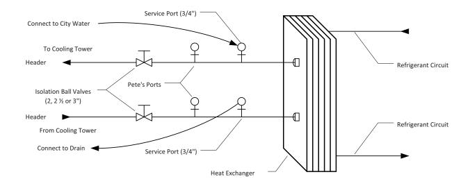
Figure 26 - In Place Cleaning Arrangement
