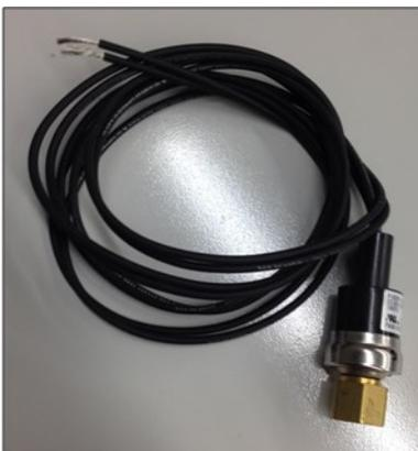
**High Pressure Switch:** The high pressure switch is an automatic reset control that senses compressor discharge line pressure. It opens at 400 PSIG and closes at 300 PSIG.
