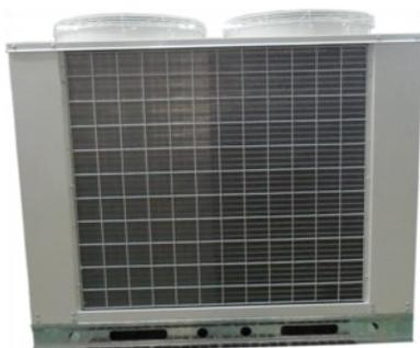
**Condenser Coil:** The air-cooled condenser coil is made of copper tube with an aluminum fin construction. The coil is protected by a painted, metal condenser grille.
