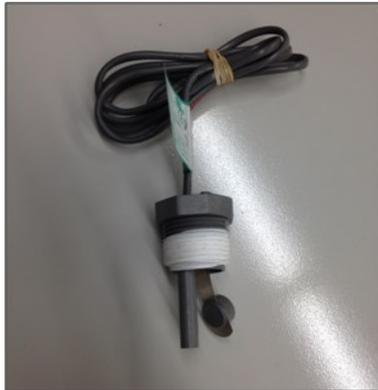
**Flow Switch:** The flow switch senses liquid solution flow. The paddle of the switch is inserted through a fitting into the pump discharge line. Liquid solution flow deflects the paddle and closing the switch. The flow switch is position sensitive. The arrow ↑ on the switch must point in the direction of liquid solution flow. Maximum flow is not to exceed 28.8GPM
