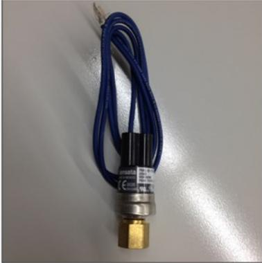
**Low Pressure Switch:** The low pressure switch is an automatic reset that senses compressor suction line pressure. In early production models, it opens at 40 PSIG and control closes at 80 PSIG. In the latest productions models, it opens at 10 PSIG and control closes at 25 PSIG.
