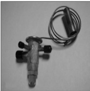
**Thermal Expansion Valve:** Multiaqua chillers are equipped with thermal expansion valves. The valves feature a liquid charged sensing bulb for consistent superheat at various load conditions.
