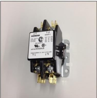
**Compressor Contactor:** The compressor contactor energizes the compressor through the two or three normally open contacts. The contactor coil operates by closing the contacts when energized by 24 vac.
