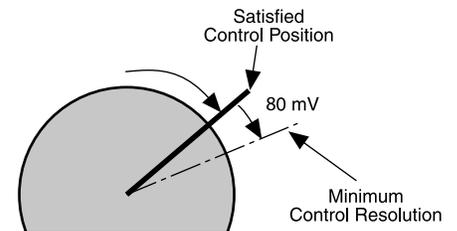
**EF Actuator responds to a 200 mV signal when reversing direction from stop position.**
