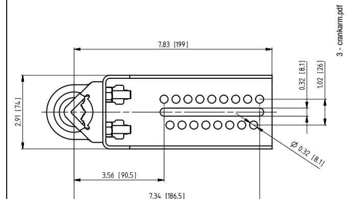
**NOTE:** The KH-EFB crank arm is designed to attach itself with the K9-2 clamp. The supplied rod must be used when the actuator is not direct coupled onto a shaft.
