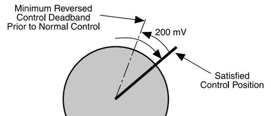
**Note:** Resolution is a percentage of operating range. 1% in one direction, 2.5% when changing direction. 2-10 VDC control example shown above.
