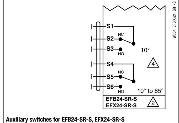
Auxiliary switches for EFB24-SR-S, EFX24-SR-S
