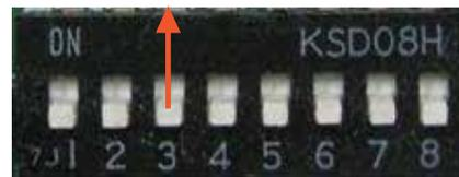
\*For Gen 4 Multi V floor standing indoor units, DIP switches 1, 2, 6 through 8 must be set to OFF. These DIP switches are used for other models.
