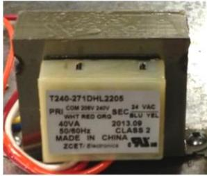
**Control Transformer:** The control transformer is rated at 24 vac, 40 va (1.6 amps @ 24vac).
