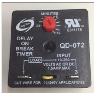
**System Delay Timer:** The refrigerant timer is a 24 vac, 5-minute delay on break timer. The normally closed contacts of the timer energize the compressor contactor through the chilled liquid solution control. When the chilled liquid solution control contact opens, the timer delays by opening its contact for 5 minutes before resetting to the closed position.
