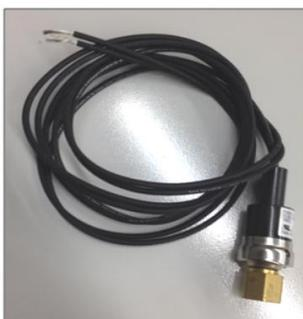
**High Pressure Switch:** The high pressure switch is an automatic reset control that senses compressor discharge line pressure. It opens at 400 PSIG and closes at 300 PSIG.
