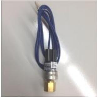
**Low Pressure Switch:** The low pressure switch is an automatic reset that senses compressor suction line pressure. In early production models, it opens at 40 PSIG and control closes at 80 PSIG. In the latest production models, **it opens at 10 PSIG and control closes at 25 PSIG.**
