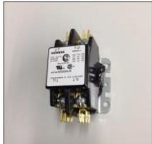
**Compressor Contactor:** The compressor contactor energizes the compressor through the two or three normally open contacts. The contactor coil operates by closing the contacts when energized by 24vac.
