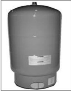
**Supply Storage Tank:** A supply storage tank must be used in a system with less than 50 gallons or 5 gallons per ton - whichever is greater-of liquid solution. The tank prevents rapid cycling of the compressors and acts as a reservoir for chilled liquid solution.
