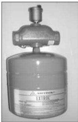
**Expansion Tank and Air Scoop:** The expansion tank and air scoop assembly is used to compensate for the expansion and contraction of liquid solution in the system. The air scoop eliminates air entrained in the liquid solution.
