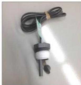
**Flow Switch:** The flow switch senses liquid solution flow. The paddle of the switch is inserted through a fitting into the pump discharge line. Liquid solution flow deflects the paddle and closing the switch. The flow switch is position sensitive. The arrow ↑ on the switch must point in the direction of liquid solution flow. **Maximum flow is not to exceed 14.4 GPM**
